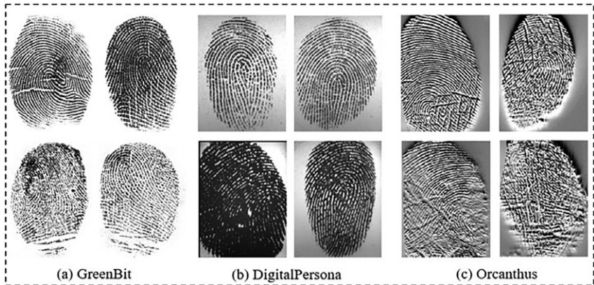
Fig. 17 Fingerprint samples of live fingerprints (above) and fake (below). Fingerprints acquired from three different sensors: GreenBit, DigitalPersona and Orcanthus. Source: LivDet 2017 fingerprint database .
