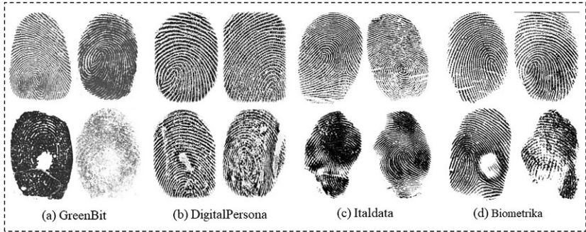
Fig. 16 Fingerprint samples from live (above) and fake (below). Fingerprints acquired with four different sensors: (A) GreenBit. (B) DigitalPersona. (C) Italdata. (D) Biometrika. Source: LivDet 2015 fingerprint database .
