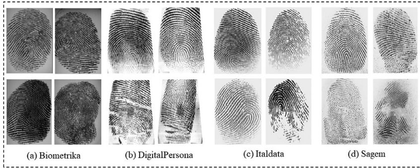
Fig. 14 Fingerprint samples from live (above) and fake (below). Fingerprints acquired with four different sensors: (A) Biometrika. (B) DigitalPersona. (C) Italdata. (D) Sagem. Source: LivDet 2011 fingerprint database .
