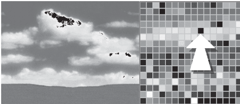
Figure 2.3 Bckgnd.bmp from Figure 2.2 with one palette entry changed to black
