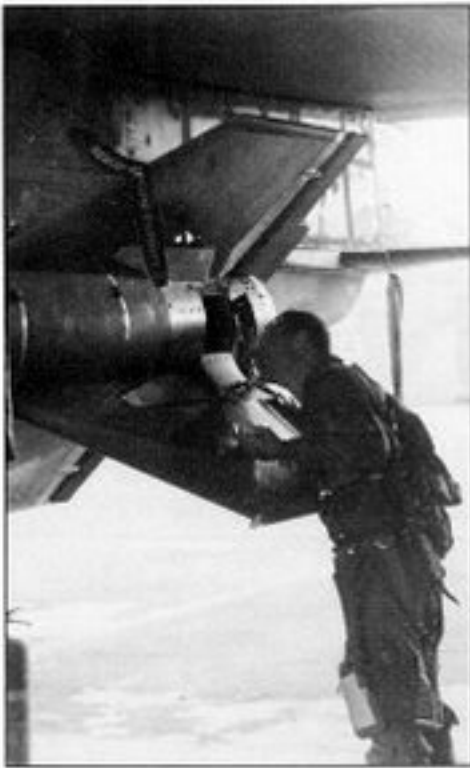
A Baz navigator examines the steering mechanism in the tail of the GBU-15 affixed to the left wing stores pylon of his Baz prior to departing Tel Nof for Tunis on 1 October 1985
