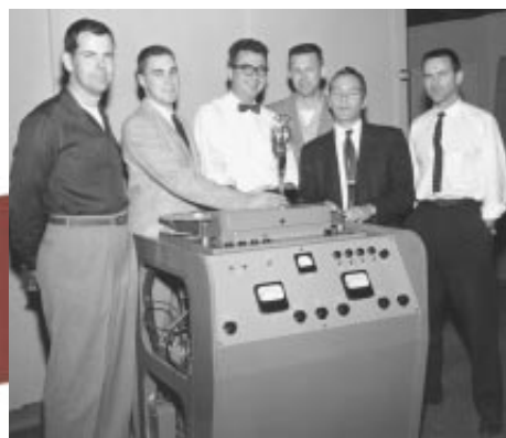
1956 VR-1000, the first commercial videotape recorder, is demonstrated in prototype by Ampex. The large, complex equipment uses tape that is five centimeters (two inches) wide.
