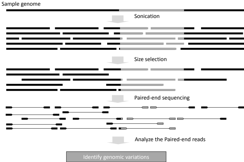
FIGURE 7.7: The illustration of the NGS protocol for whole genome sequencing. In this example, a gray-colored sequence is inserted into the genome. The two boundaries between the black and gray colored sequences are called breakpoints. Paired-end reads that cross the breakpoints are called anomalous paired-end reads. The reads that overlap with the breakpoints are called split-reads. (Split-reads are reads that contain both black and gray colored sequences while anomalous paired-end reads are paired-end reads that contain both black and gray colored sequences.)
