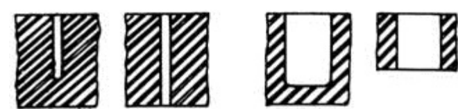
Fig. 8.6 Shallow, wide holes are preferred.
