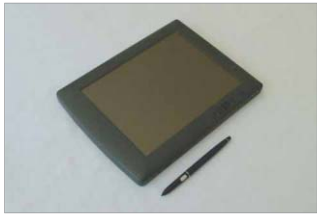
Figure 2. Microsoft's proof-of-concept Tablet PC based on Transmeta's early TM5800 processor (1999).
