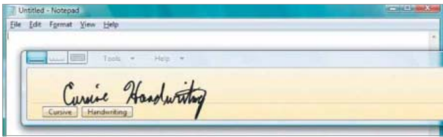
Figure 1. Tablet PC input panel. The input panel lets users write directly on the Tablet PC.
