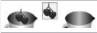
Figure 6-6: Transparent copy blit of strawberry sprite and blender image background to achieve composite result of both
