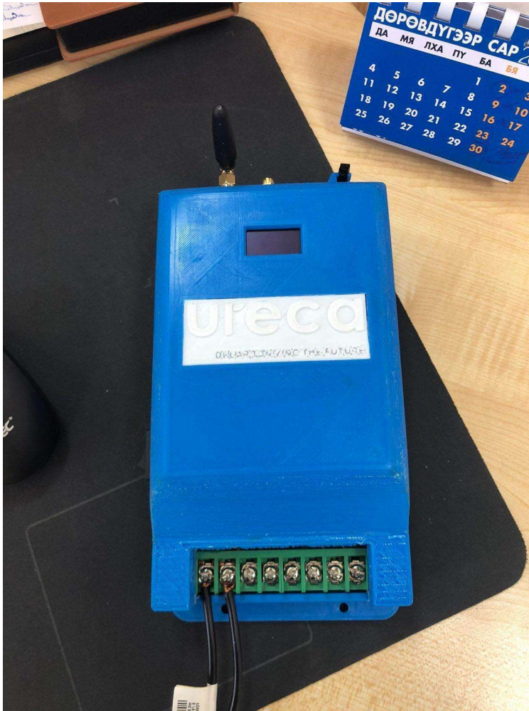
Photo 5. Assembled URECA meter with a-3D printed case
