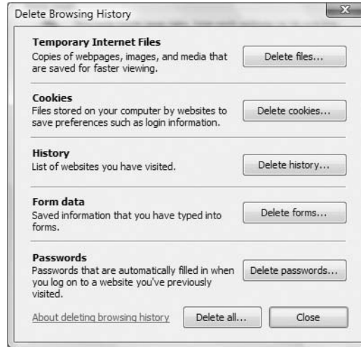
Figure 2-21: Dialog box in Internet Explorer that you use to remove files so that they are refreshed with new ones
