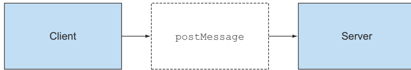
Figure D.6 postMessage allows two <iframe> tags from different origins to communicate.
