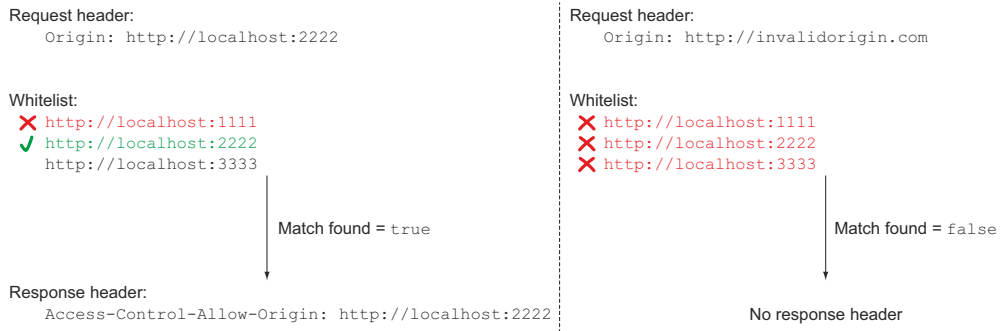
Figure 6.3 Example of using a whitelist to find a valid and an invalid Origin header
