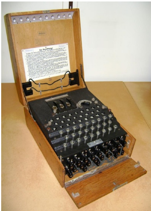
Figure 2-1. The German Wehrmacht Enigma (Copyright © 2014 Dirk Rijmenants) 9
