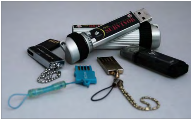
Figure 2.3 UFDs, ranging in physical size (tiny blue model and large Survivor model with waterproof case both hold 8 GB of data)
