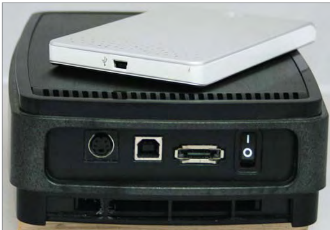
Figure 2.4 Two external hard disks: 160 GB 2.5" USB mini-jack type on top of 1.5 TB 3.5" USB Type B jack
