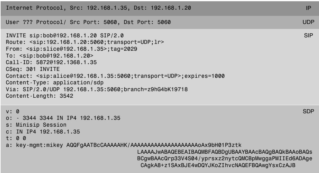
FIGURE 6.4 Use of MIKEY in SIP for key negotiation.
