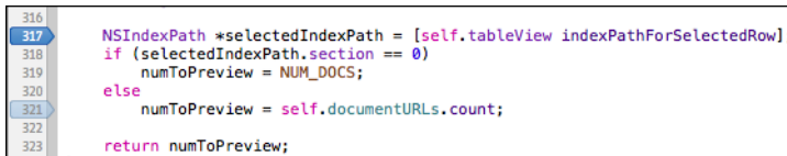
Figure 5-2: Setting breakpoints on specific lines with the mouse. Deactivated breakpoints are shaded a lighter gray.
