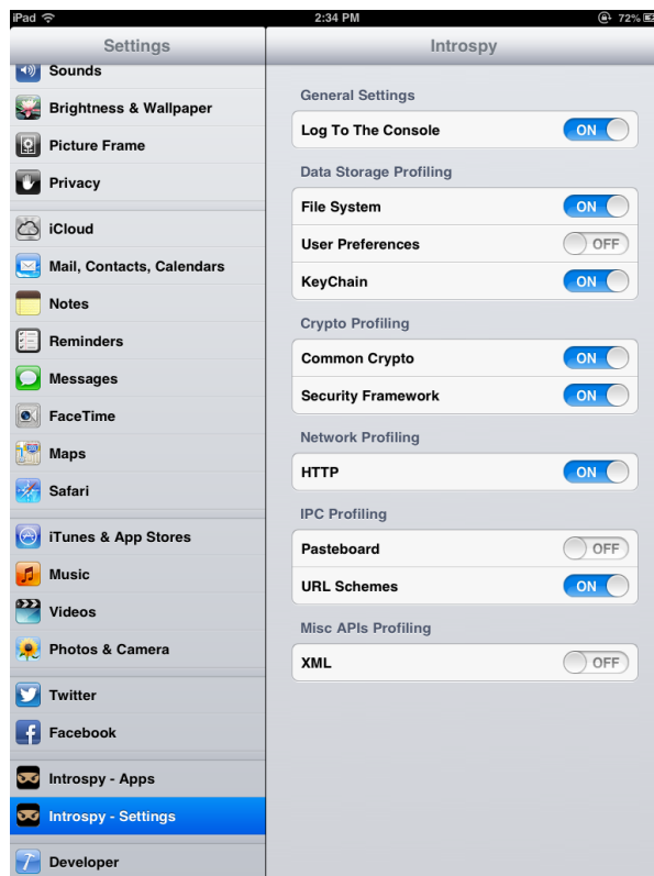
Figure 6-7: The Introspy settings screen. You can select which applications are profiled on the Apps tab.
