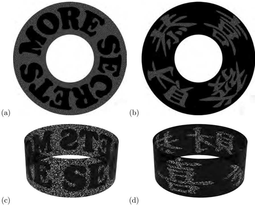
FIGURE 3.23 Transforming circle shares (a) and (b) into cylinder counterparts (c) and (d), respectively.
