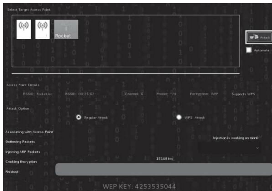
Figure 119 - WEP Key Cracking
