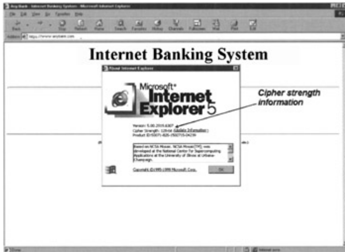
Figure 5.7: Viewing the browser's encryption strength. (Microsoft IE5 screen shot reprinted by permission of Microsoft Corporation.)
