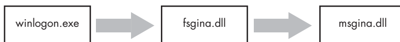
Figure 11-2: Malicious fsgina.dll sits in between the Windows system files to capture data.
