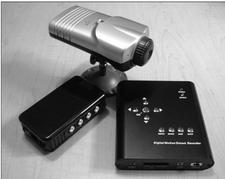
Figure 9-11 Examples of video surveillance devices available to home users. Clockwise from top: IP-enabled video camera, a two-camera DVR with built-in motion detection, and a TCP/IP network video server that supports four analog cameras/video sources. All items retail for less than U.S. $150.
