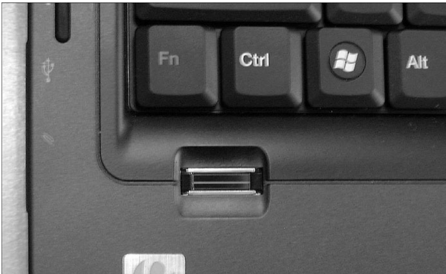
Figure 9-10 A fingerprint reader (horizontal bar located beneath Fn and Ctrl keys) found on the author's Gateway laptop
