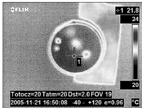
Figure 9-9 A thermal camera shows thermal fingerprint residue (small dots) on the keys of a safe keypad (large circular ring). The intensity of the dot indicates the order the keys were pressed. (Courtesy: http://lcamtuf.coredump.cx/tsafe/ )
