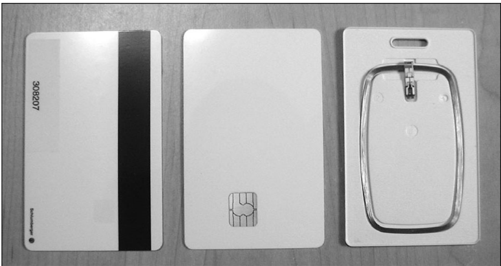
Figure 9-5 Common identification credential cards: magnetic stripe, smartcard, and radio frequency identification (RFID) (with cover removed)
