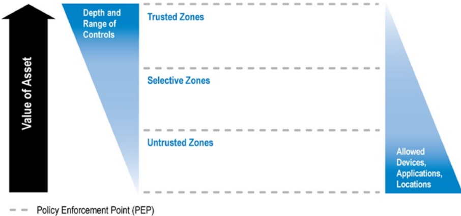
Figure 7-2. As the value of an asset increases, the depth and span of controls increase, while the number of allowed devices, applications, and locations decrease. Source: Intel Corporation, 2012
