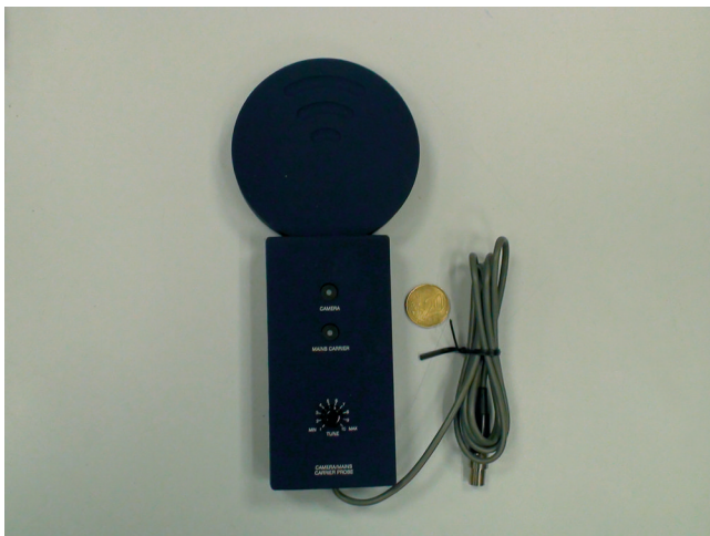
Figure 8.13 A multifunction device probe for detecting miniature cameras or mains carrier bugging devices.
