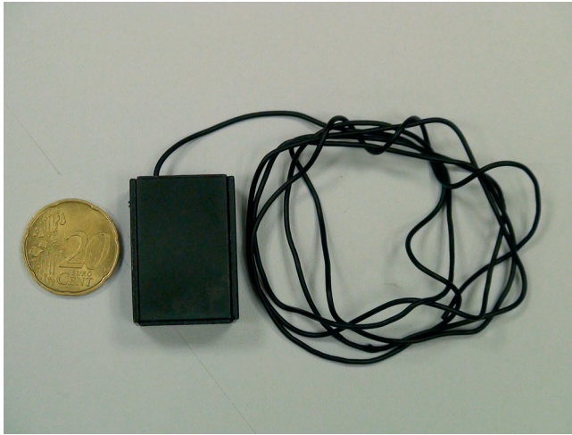
Figure 8.1 A bugging device.
