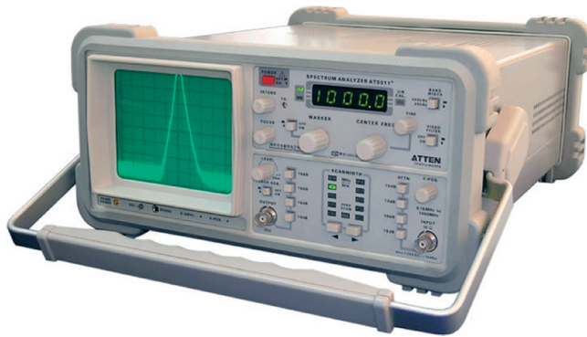
Figure 8.9 Spectrum analyser showing in detail the emission–frequency–intensity curve of an electromagnetic source.
