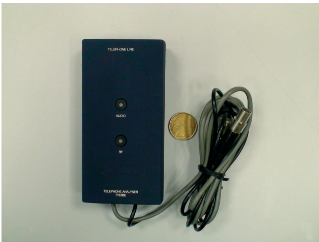
Figure 8.15 A multifunction device probe for analysing telephone lines for detecting relative bugging devices.
