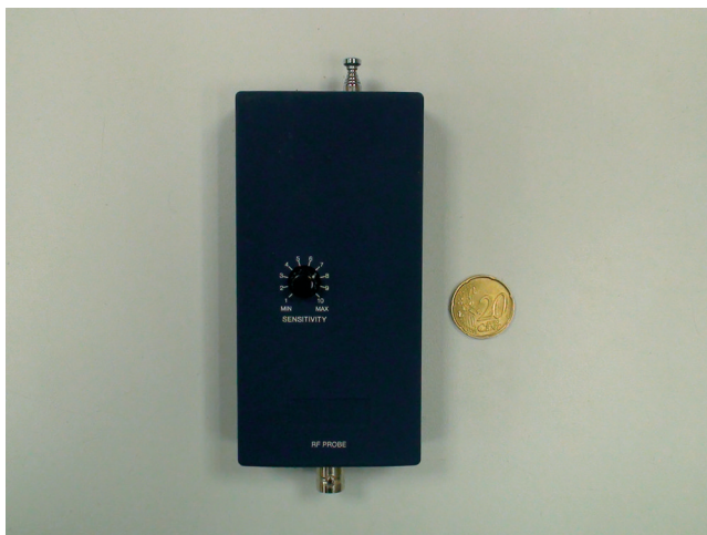
Figure 8.11 A multifunction device probe for detecting radio frequency or microwave bugging devices.
