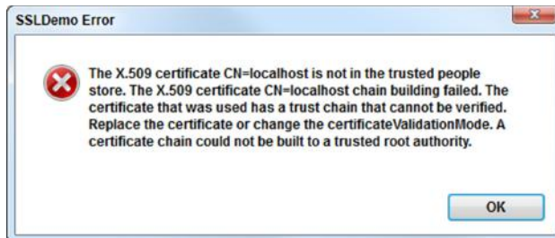
Figure 8-4: Exception is thrown by SSLDemoClient when CA root certificate is not found
