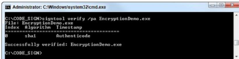
Figure 9-11: Verifying the code signature using SignTool
