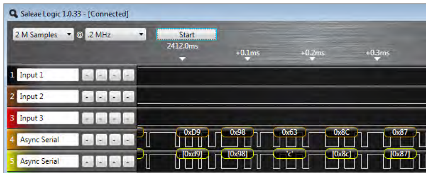
Figure 13-17: Saleae Logic Analyzer byte display
