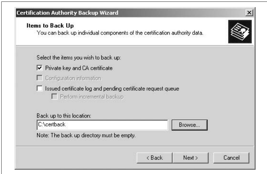
Figure 6-11. Backing up key data for a CA
