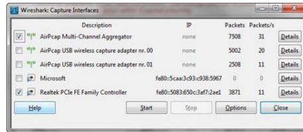
Figure 75. The Interfaces List shows traffic activity without capturing traffic
