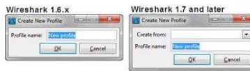
Figure 164. Make new profiles based on existing ones in more recent versions of Wireshark
