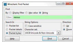
Figure 49. You can find packets based on display filter, hex value or string
