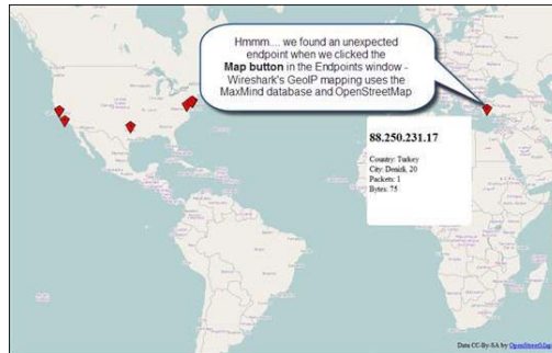
Figure 129. GeoIP can be run from the IPv4 or IPv6 tab of the endpoints window[ http-wireshark-ipv6.pcapng ]
