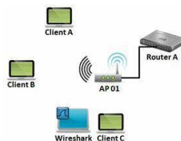
Figure 73. Place Wireshark close to the client to analyze traffic from the client's perspective
