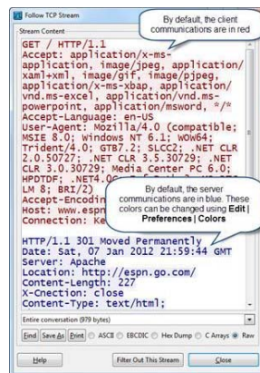
Figure 110. Stream coloring is seen when you reassemble UDP, TCP or SSL streams [http-espn2011.pcapng]
