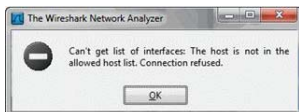
Figure 78. The Wireshark host is not listed in the <host_list> file on the system running rpcapd
