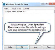
Figure 36. User Specified Decodes correspond to the Decode As setting and can now be saved
