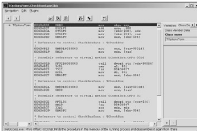
Figure 2.1: The DeDe program window displaying the disassembled code of a button-click event in an application
