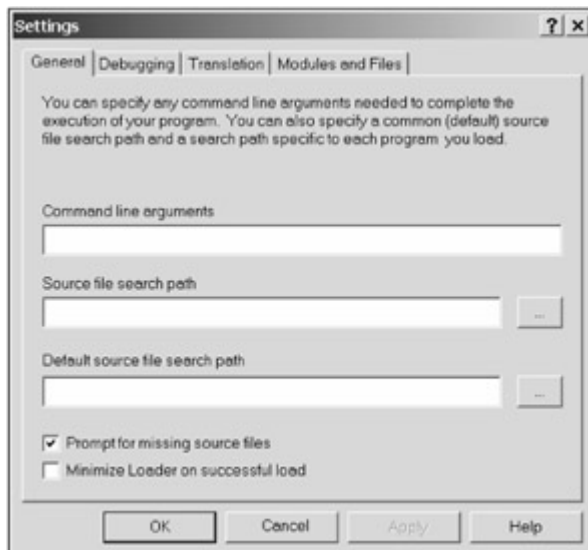
Figure 4.3: The Settings window allows you to set the loading parameters for the modules to be debugged
