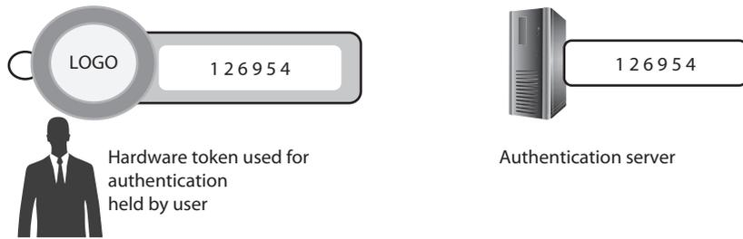
**Figure 2-5** Token used for token-based authentication
