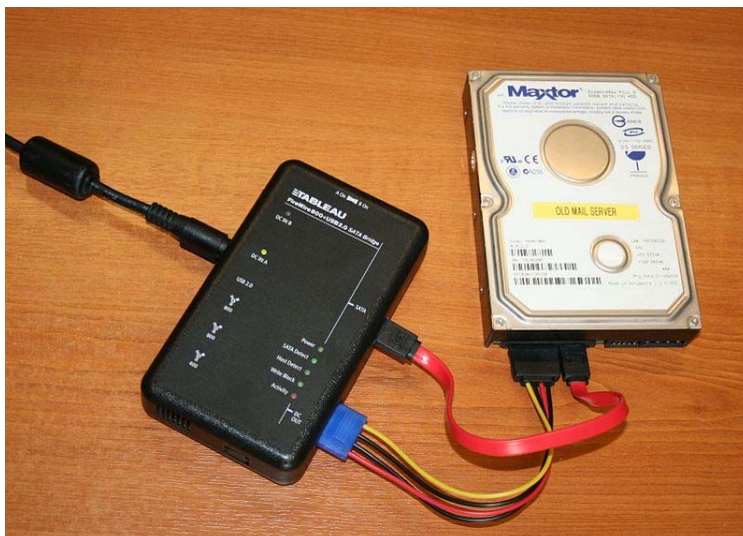
FIGURE 6.1 A hard drive attached to a Tableau portable forensic write blocker
