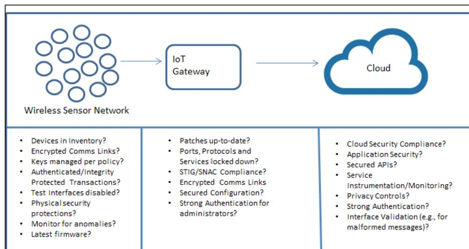
We can evaluate collected security-relevant data by considering an IoT architectural model of WSN endpoints transmitting data to a protocol gateway, then that gateway passing the data to the cloud. Once in the cloud, we can leverage the capabilities of the **cloud service provider (CSP)** to capture data between application endpoints supporting the IoT sensors. For example, within Amazon we can leverage AWS CloudTrail to monitor API calls to the cloud.
