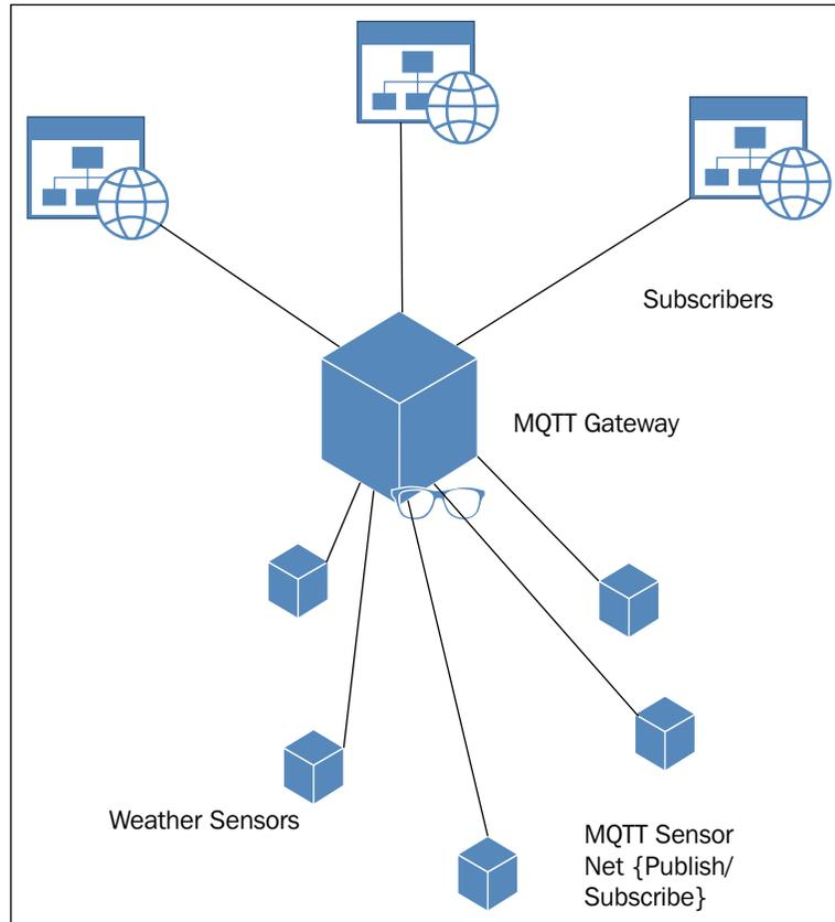
This neatly supports a variety of communication use cases, wherein sensors MQTT-publish their data to a broker and the broker passes them on to other subscribing systems that have an interest in consuming or further processing the sensor data. Although MQTT is primarily suited for use over TCP-based networks, the **MQTT For Sensor Networks (MQTT-SN)** specification provides an optimized version of MQTT for use within **wireless sensor networks (WSN)**.
