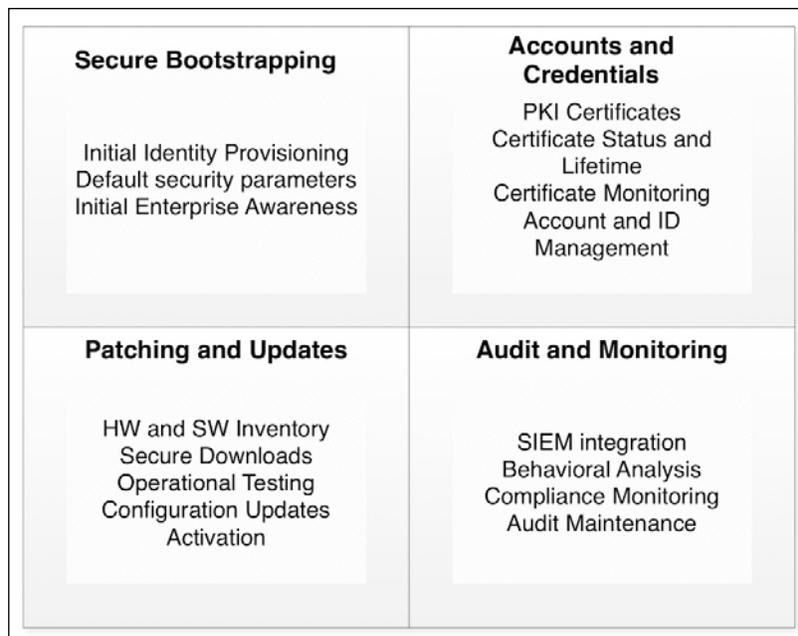
Artifacts from threat modeling, PIA, SIA, and compliance analysis should be used as inputs into an overarching IoT security system design. For example, during bootstrap (initial provisioning and connection) of an IoT device into a larger enterprise or home network, there may be security-critical processes related to treatment and handling of default passwords, technical controls to enforce the creation of new passwords, one-time symmetric keys, and so on.
