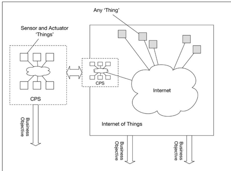
In other words, it is worthwhile to think of the IoT as a superset of CPS, as CPS can be enveloped into the IoT simply by connectivity to the Internet. A CPS is generally a rigorously engineered system designed for safety, security, and functionality. Emergent enterprise IoT deployments should take lessons learned from the engineering rigor associated with CPS.
