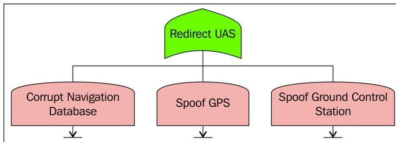
You will notice the two well-known logic operator symbols for AND (smooth and rounded top) and OR (pointy top). The root node, entitled **Redirect UAS** represents the end objective and is made up of an OR operator. This means that any one of its children can satisfy the end goal. In this case, the attacker may redirect the aircraft by any of the following methods:
