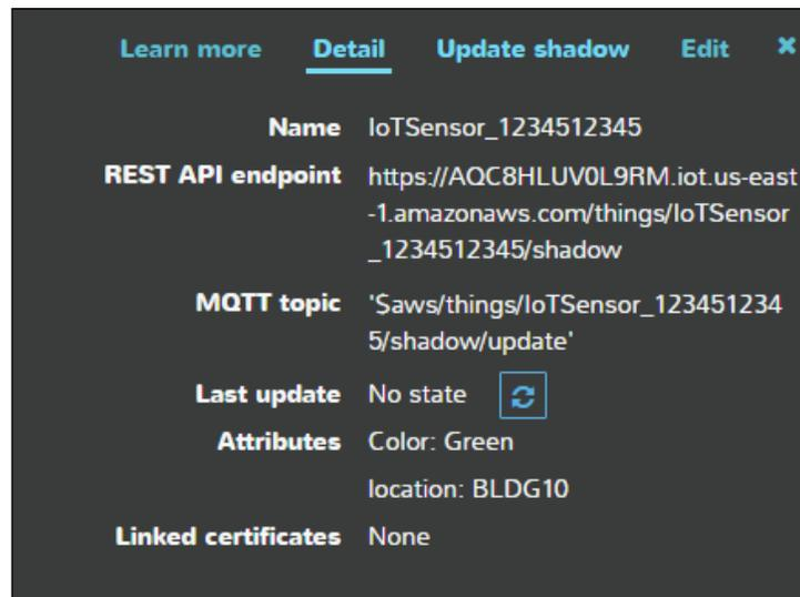
The AWS Thing Shadow is an intermediary between a controlling application and the IoT device. Thing shadows leverage the MQTT protocol with predefined topics that can be used to interact with the service and devices. MQTT messages that are reserved for the Thing Shadow service begin with `$aws/things/thingName/shadow`. The following are the reserved MQTT topics that can be used to interact with the shadow (<https://docs.aws.amazon.com/iot/latest/developerguide/thing-shadow-mqtt.html>):
