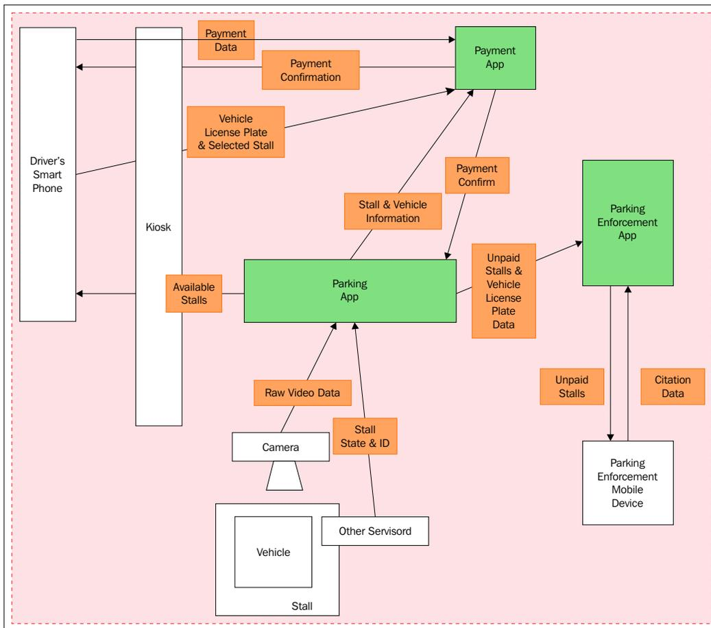
Once data flows have been thoroughly examined, you can begin to catalogue the various physical entry points into the system and the intermediate and internal gateways through which data flows. Also identify trust boundaries. The entry points and trust boundaries have an enormous security bearing as you identify overall threats associated with the system:
