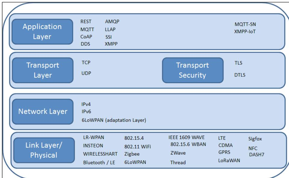
This figure provides a view into some of the better-known protocols that can be implemented by IoT devices to form a complete communications stack.
