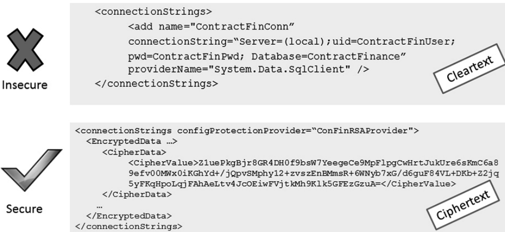
Figure 4.7 – Insecure and secure ways of storing connection strings in a configuration file
