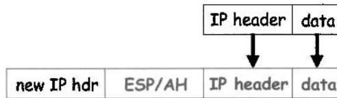
Figure 10.17: IPSec Tunnel Mode
