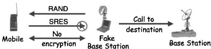
Figure 10.26: GSM Fake Base Station
