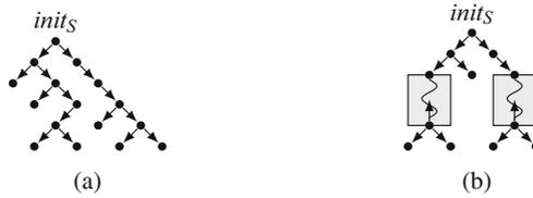
**Fig. 13.9** Execution model. In **(b)** the *shaded boxes* show single-path (concrete) execution through the simulation model due to MMIO. **(a)** Fully symbolic execution. **(b)** Selective symbolic execution
