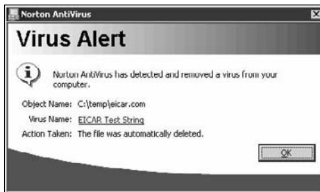
Figure 13-11: Using the EICAR test string to test antivirus software.
