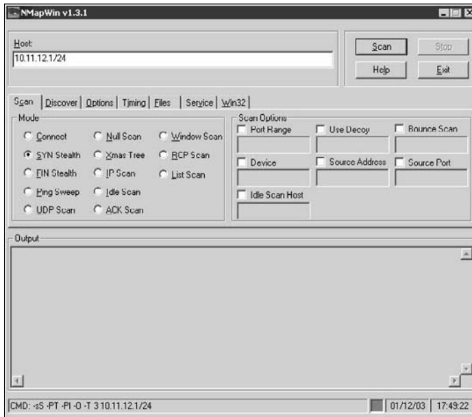
Figure 8-3: In-depth port- scanning options in NMapWin.
