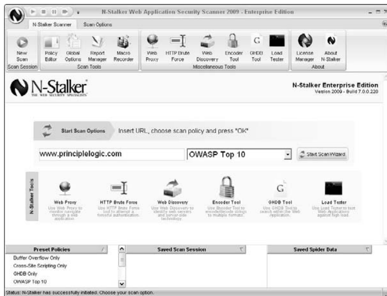
Figure 14-9: Using N-Stalker Web Application Security Scanner to check a wide range of basic Web application vulnerabilities.
