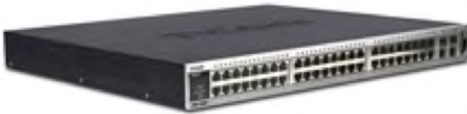
Figure 10–3. D-Link 48 port managed switch
