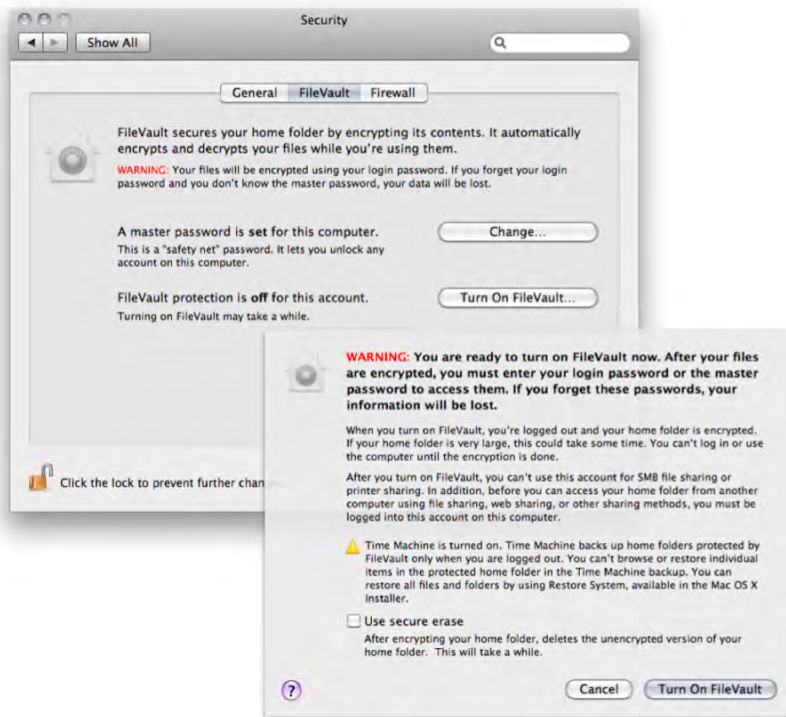
Figure 9–12. The FileVault tab found in the Security system preference pane (back), and associated dialog when enabling the feature (front).
