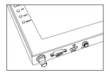
3G-SDI – Serial Digital Interface Connection VGA – Video Graphics Array DE15 Connection HDMI – High-Definition Multimedia Interface Input Connection Power Port – 12-24v Input
