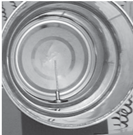
Figure 8-8 Antenna wire extruding inside the antenna body (photo courtesy of Julian “HammerJammer” Ho)
